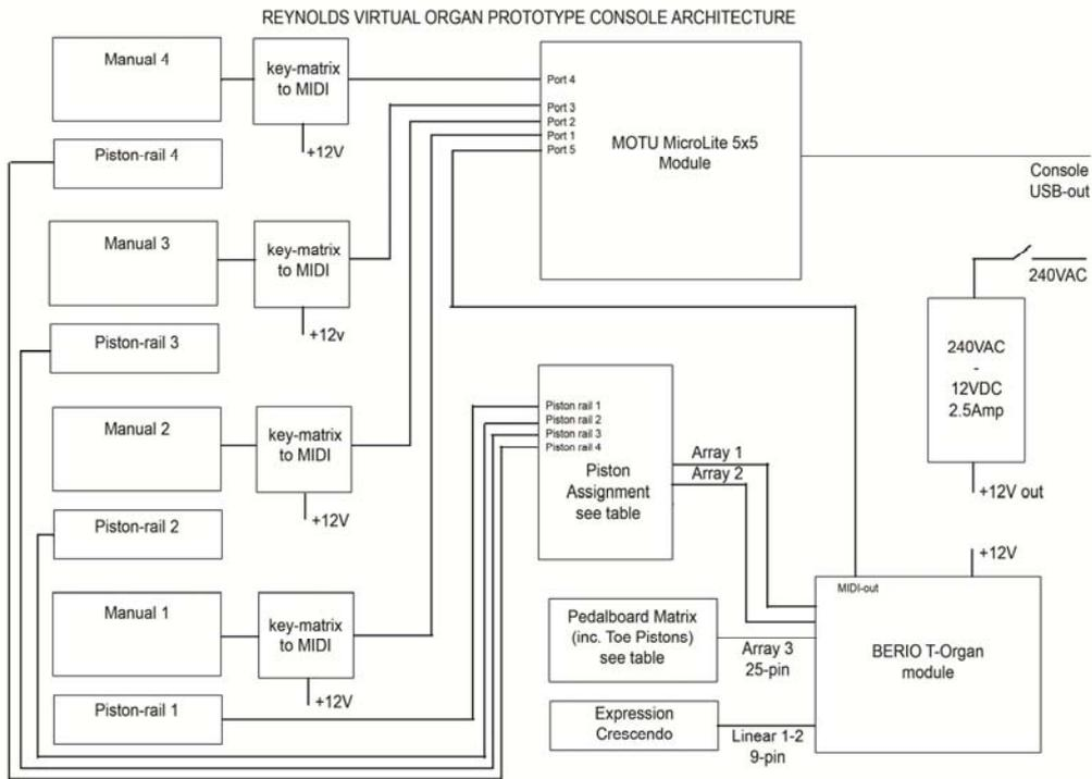
Figure 2: Console Architecture (note: common earth and power negative)
