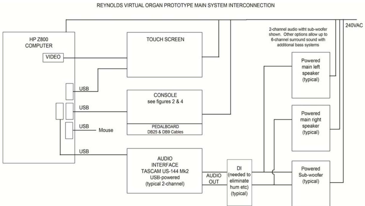
Figure 3: System Interconnections (note: USB assignments as viewed from rear of computer)
