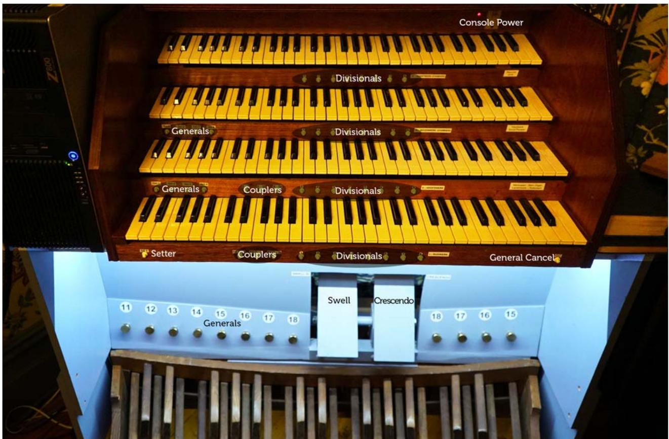
Figure 1: Console showing thumb & toe-pistons and expression pedal layouts (typical – This arrangement specific to Laurenskirk Rotterdam Main Organ – Sonus Paradisi)
